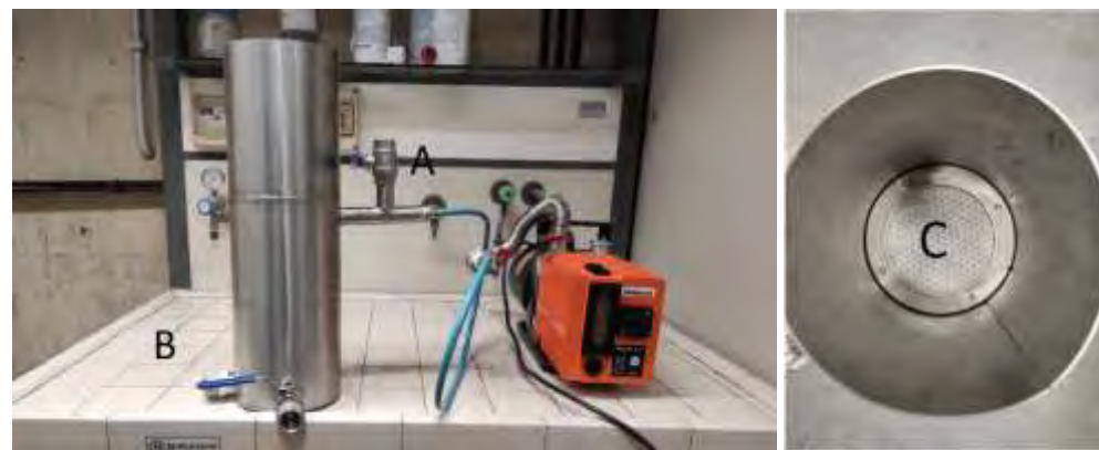
Experimental filter for the removal of suspended solids from vegetation water: A) hydraulic valve connecting the lower chamber with a vacuum pump; B) filtered water drain valve. Right: Top vision of the filter before adding the layer of straw filtering material: C) the support technical sheet.
